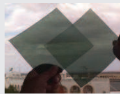
Fig. 4a: If the filters have the same orientation, light passes through.
