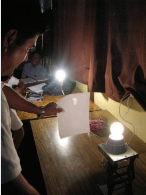
Fig. 16: Oil slick photometer, between two light bulbs.
